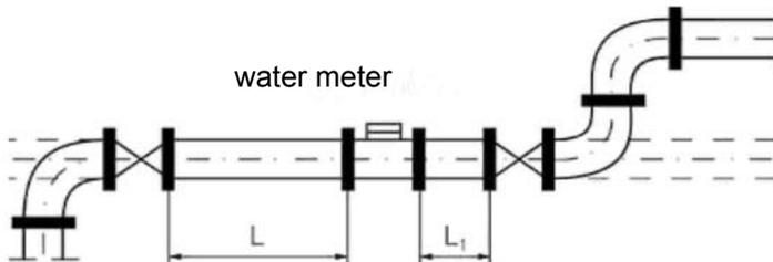
6.7 Water meter should not be under risk of excessive strain caused by pipelines and equipment. If necessary, install it on a pedestal or in a grip. What is more, the pipes connecting on the inlet and outlet side should be adequately fastened, so that no part of the system is dislocated by the water when the water meter is deinstalled or disconnected from one side.
